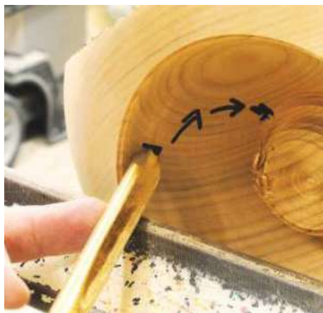
▲ Pic.29 Keeping the bevel in contact with the wood requires the tool to be passed through the wood in this way. Start horizontal and as you go through the shape, raise the tool tip higher, then lower down as you get to the centre
